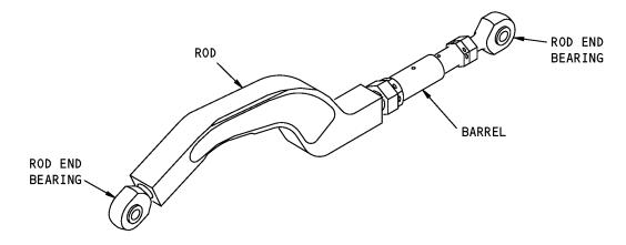
Aileron Tab Control Rod Assembly Figure 1
