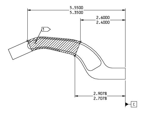
1 APPLY BMS 10-86, TYPE 1 OR TYPE 2, ABRASION RESISTANT TEFLON COATING, COLOR BAC707 GRAY (F-14.9625)
