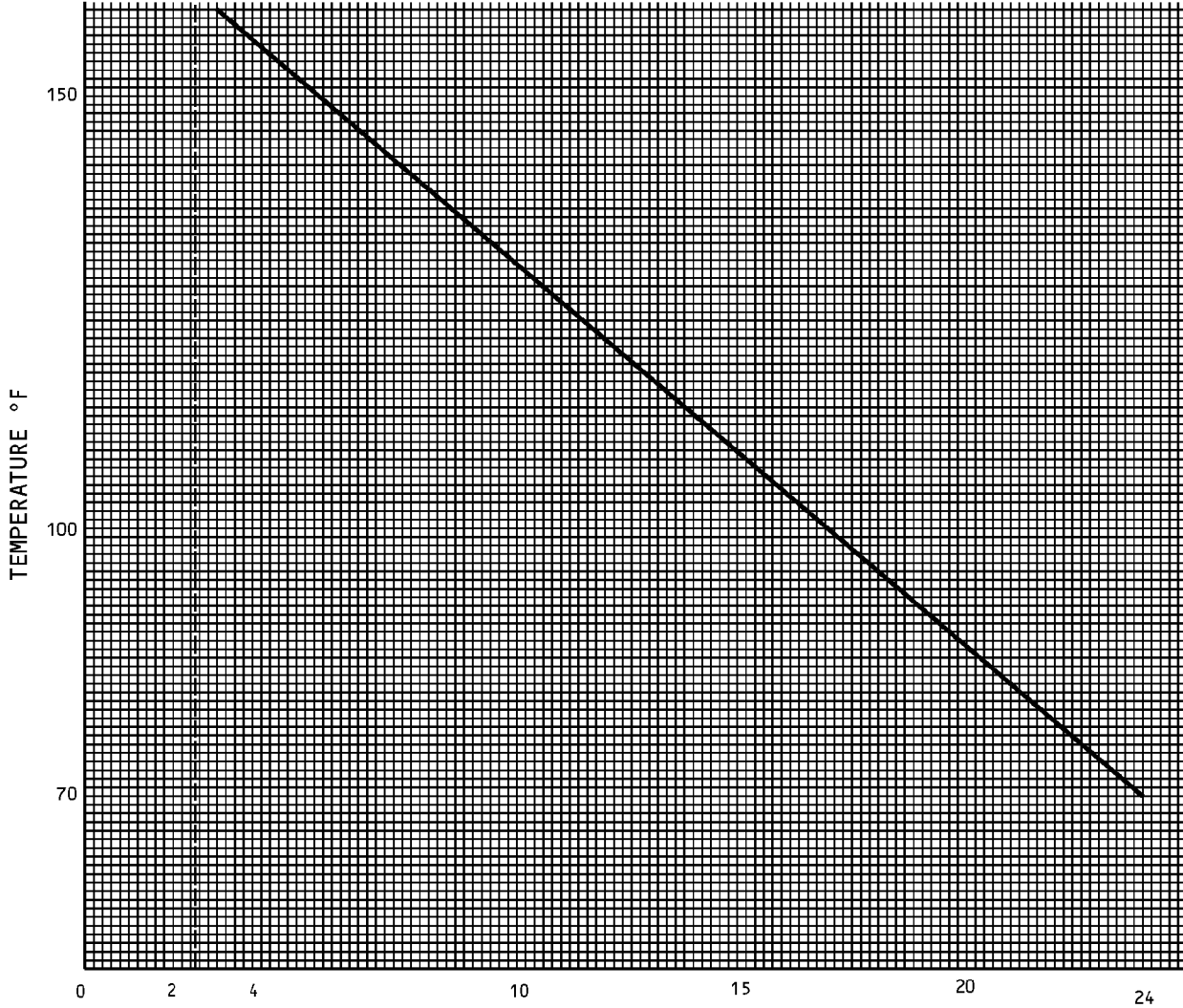
TIME IN HOURS (CURE CURVE FOR EA 9330 A/B ADHESIVE)
