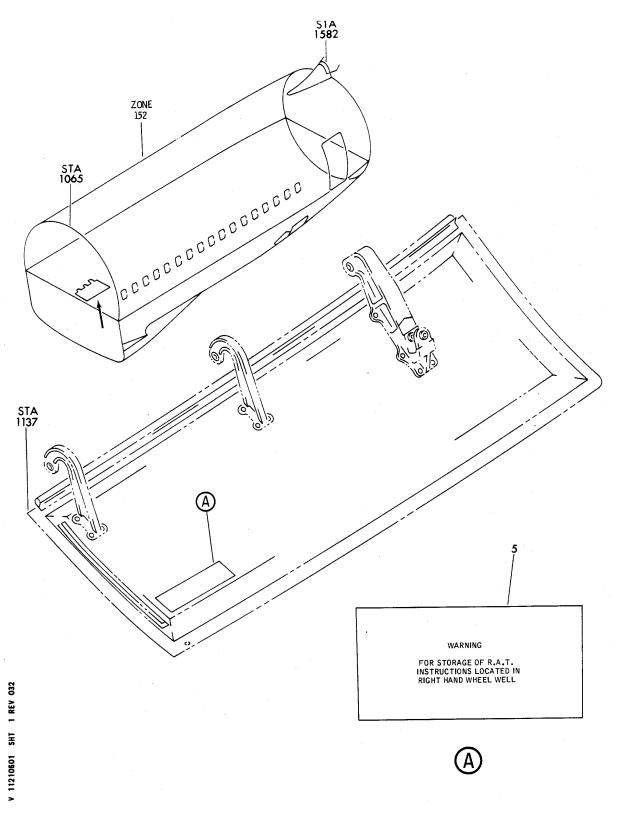
DOOR ASSY-RAM AIR TURB AFT FAIRING (PLACARDS AND MARKINGS ONLY) FIGURE 1
