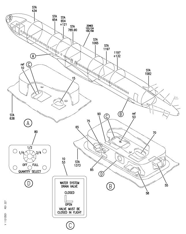
PANEL INSTL-STA 632 AND STA 1373 POTABLE WATER SYS SERVICE AND DRAIN (PLACARDS AND MARKINGS ONLY) FIGURE 1
