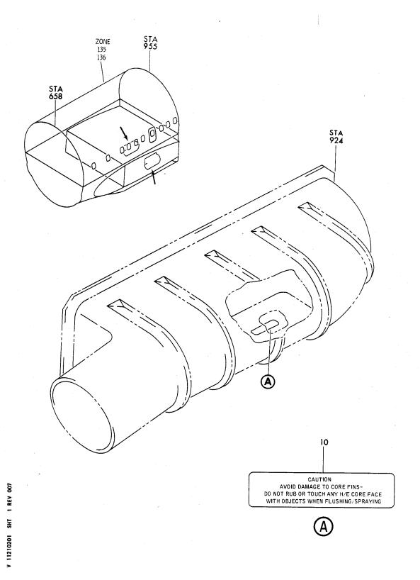
DUCT ASSY-RAM AIR SYS HEADER (PLACARDS AND MARKINGS ONLY) FIGURE 1
