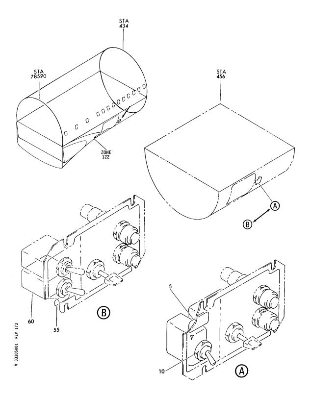
PANEL ASSY-LARGE CARGO DOOR ACTUATION CONT (P43) (CARGO AND SERVICE COMPARTMENT LIGHTS ONLY) FIGURE 1
