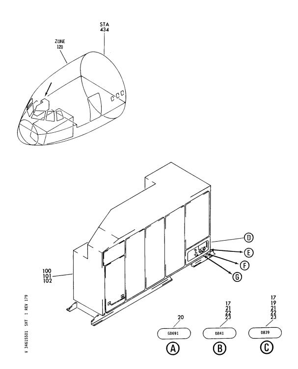
EQUIPMENT ASSY-MAIN PWR DISTR P6 PNL (FLIGHT MANAGEMENT COMPUTER SYSTEM ONLY) FIGURE 1 (SHEET 1)
