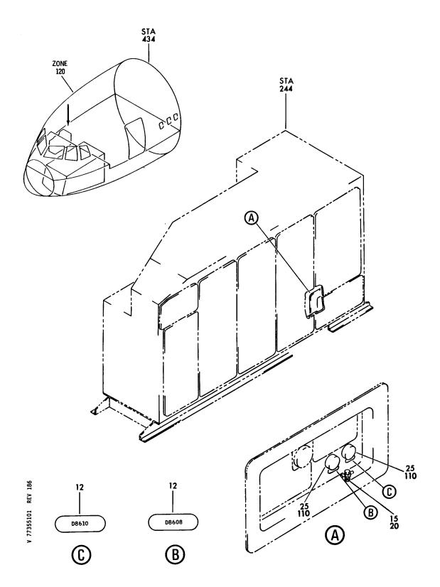
EQUIPMENT ASSY-MAIN PWR DISTR P6 PNL (ELECTRONIC PROPULSION CONTROL SYSTEM ONLY)
