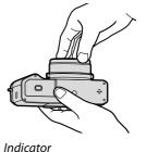
2 Attach the adapter ring. With the indicator facing up as shown, align the projections of the adapter ring with the grooves on both sides of the lens and install the adapter ring (①), and then rotate the outside of the adapter ring to secure it (②).
