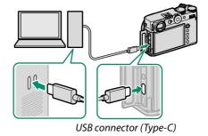
① The USB cable must be no more than 1 m (3.3 ft.) long and be suitable for data transfer.
