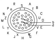
CONNECTOR PART NO.: MS3102A28-12P MATING CONNECTOR: MS3106A28-12S
