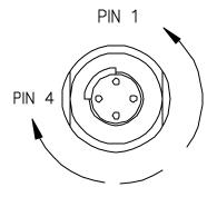
CONNECTOR PART NO.: XSE-4-BCR MATING CONNECTOR: XSE-4-CCP
