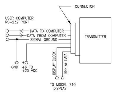
Proper connection requires identifying the correct output pins on the computer RS-232 port and on our transmitter output connector.
