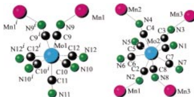
Figure 2. Environment of the Mo1 (left) and Mo2 sites (right) in 1 . The color code is the same as for Figure 1. Selected mean interatomic distances [Å] and angles [°]: Mo1-C 2.148, Mo2-C 2.166; Mo1-C-N 176.8, Mo2-C-N 176.8.
