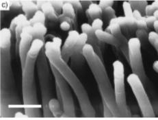
Figure 4. SEM micrographs taken from a nanotube electrode, which was partially inserted into an aqueous solution of  $NaClO_4$  (0.1M) containing pyrrole (0.1M) after three cycles between -0.6 and  $0.6\,V$  (scan rate  $25\,mV\,s^{-1}$ ). The images were taken at a) the air/electrolyte solution interface, b) the same position as a) at a higher magnification, and c) immersed in the electrolyte solution. Scale bars are 2 (a) and 1  $\mu$ m (b, c).
