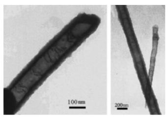
Figure 3. Typical TEM images of the CP-NT coaxial nanowires formed from the cyclic voltammetric method, the images are in the tip region (left) and on the wall (right).
