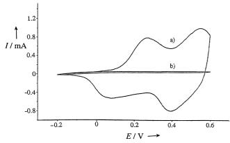
Figure 5. Cyclic voltammograms of a) the polyaniline-coated CP-NT coaxial nanowires and b) the bare aligned carbon nanotubes. Measured in an aqueous solution of  $1 \text{ M} \ \text{H}_2 \text{SO}_4$  with a scan rate of  $50 \ \text{mV} \ \text{s}^{-1}$ .
