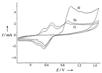
Figure 2. Electropolymerization of aniline (0.1m) in  $H_2SO_4$  (0.2 m) onto the aligned nanotube electrode. a) First cycle; b) second cycle; c) third cycle. Scan rate is 25 mV s<sup>-1</sup>
