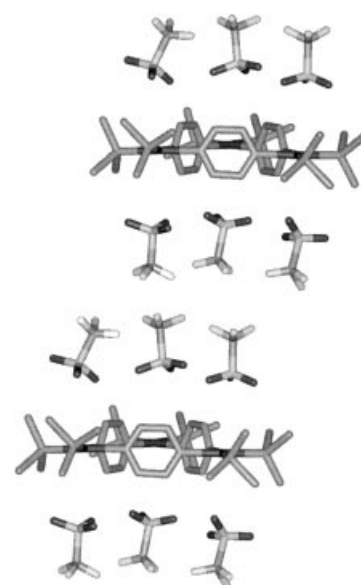
Figure 2. Stacking of 3 into staggered columns (side view; stick representation; dark portions of triflate anions represent oxygen atoms, light portions represent fluorine atoms). Protons omitted for clarity.
