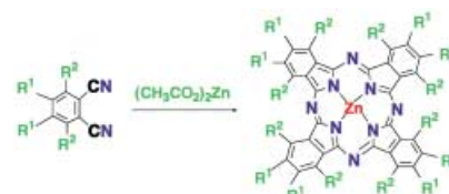
Scheme 1. Synthesis of [F_{64}PcZn(\text{acetone})_2] ( 2 ) (acetone molecules omitted); R^1 = CF(CF_3)_2 , R^2 = F .
