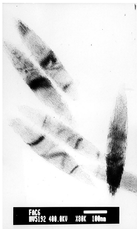
Figure 1 TEM micrograph of acicular \alpha -Fe 2 O 3 nanoparticles as prepared.
