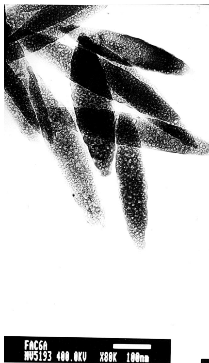
Figure 2 TEM micrograph of acicular \alpha -Fe 2 O 3 nanoparticles after annealing at 500 °C for 24 h.
