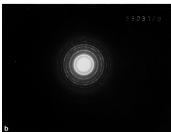
Figure 3 (a) Transmission electron micrograph of specimen containing nickel and reduced at 660 °C for 10 min; (b) electron diffraction pattern of the same specimen.
