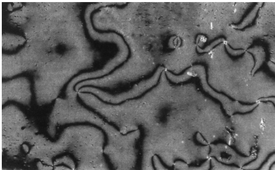
Figure 12 Photomicrograph of a ferrocenomesogen with a characteristic nematic phase exhibiting a Schlieren texture.
