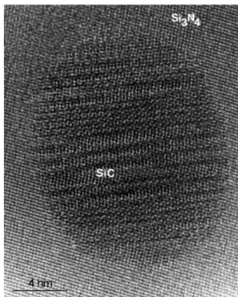
Figure 10 HRTEM image showing a SiC inclusion within a matrix made of \text{Si}_3\text{N}_4 . The material is derived from the polysilazane PHMS and subsequently annealed for 50 h at 1800 °C in a nitrogen atmosphere.
