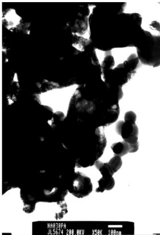
Figure 4 Transmission electron micrograph of the washed powder.
