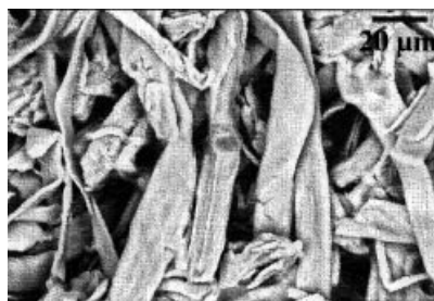
Figure 6 Scanning secondary-electron micrograph of the cellulose fibers.
