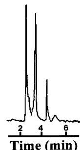
Figure 2 HPLC-THG-AA chromatogram of N -2,4-DNP derivatives of \phi\text{Hg} cysteineselenoate [retention time ( r_T ), 2.14 min], selenomethionine ( r_T , 3.49 min) and selenocystine ( r_T , 5.11 min) separated with a methanolic mobile phase containing acetic acid and triethylamine ( 0.05 and 0.8 \mu\text{l cm}^{-3} , respectively) delivered to the Nucleosil 5- \text{NO}_2 column at 0.5 \text{ cm}^3 \text{ min}^{-1} .
