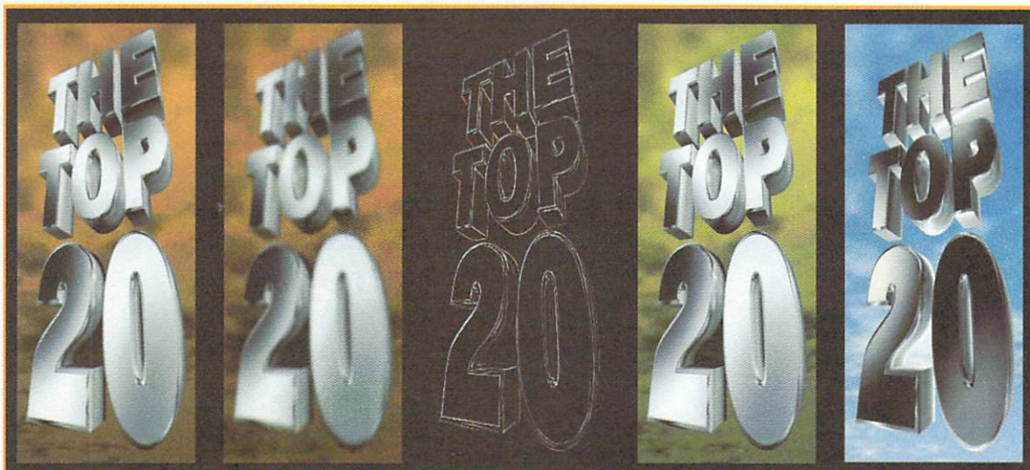
Some of the new operators that Gary's Effects provides BME with. They are: the original picture, blurred, Laplacian Edge (convolution), hue (+23°), solarized
