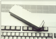
■ This is the 8-Max unit itself, an unusual-looking grey box that plugs in the Amiga's external drive port.
