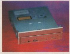
If you have an Amiga equipped with a SCSI interface, it's perfectly possible to connect a SCSI CD-ROM drive such as this Toshiba XM-4101B to your machine.
