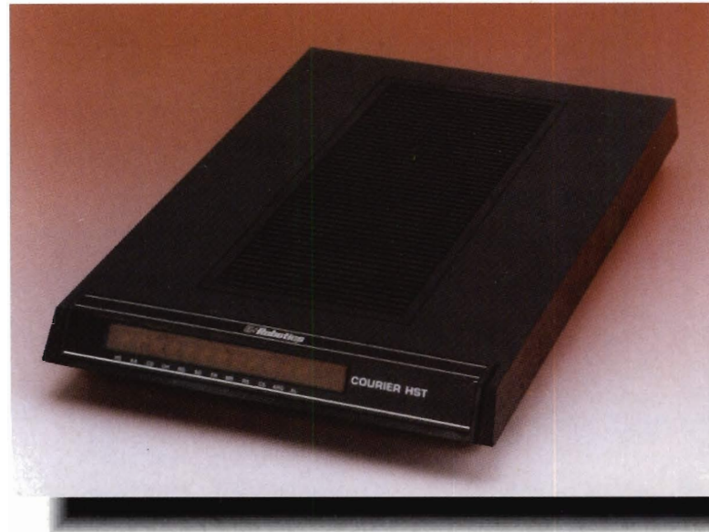
The Courier HST modem features "asymmetric modulation", MNP error control protocol levels 1 - 5, and ARQ (automatic repeat request).
