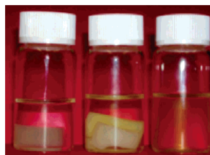
Figure 4. Aqueous degradation steps of the dimethylacrylamide-based polymeric network cross-linked with the new biodegradable cross-linker DMTLT: nondegraded disk (left sample), highly swollen and fragmented disk after a few days of degradation (center sample), and material solubilized after several weeks of aqueous degradation (right sample).
