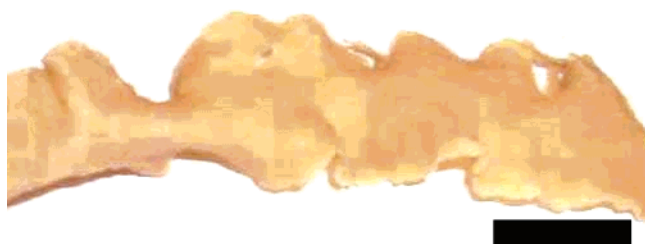
Figure 2. Wheat gluten film extrudate without salicylic acid. The bar is 5 cm long.
