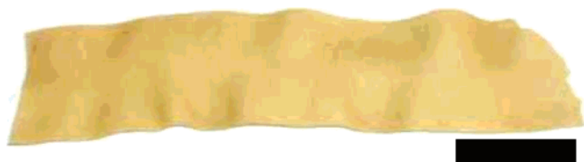
Figure 3. Wheat gluten film extrudate with 1 wt % salicylic acid. The bar is 5 cm long.
