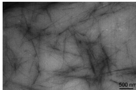
Figure 8. Transmission electron micrograph of ASA-modified cellulose whisker (DS \approx 0.02) embedded in thin polystyrene film.
