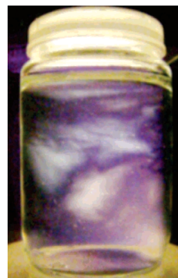
Figure 3. Transparent suspension of 0.1% cellulose microfibrils of never-dried sulfite wood pulp TEMPO-oxidized with 2.5 mmol NaClO per gram of cellulose. Observed at rest between crossed polarizers.
