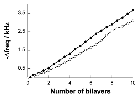
Figure 3. Typical frequency changes in QCM for the formation of (Fc-PAH/DNA) n (○) and (Fc-PEI/DNA) n films (●). The layer numbers between each integer show the deposition of Fc-PAH or Fc-PEI.
