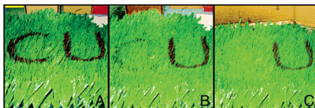
Figure 2. Removal of the logotype (colored with Red Food Color) from the artificial turf surface: (A) Dried logotype before the treatment, (B) letter "C" sprayed with 0.1M EDTA solution (using a hand-held spray bottle) and letter "U" sprayed the same way only with water, and (C) total removal of "C" with a water wash while "U" remains visible on the surface.
