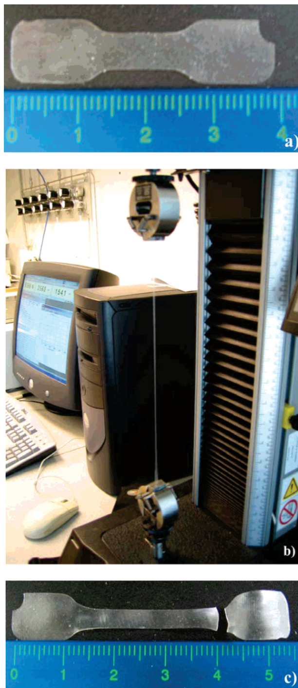
Figure 4. Photos showing the elongation and permanent set of PUU-PTMC: (a) dog-bone-shaped sample before measurement, (b) the sample elongated 2500%, and (c) permanent set of the sample.
