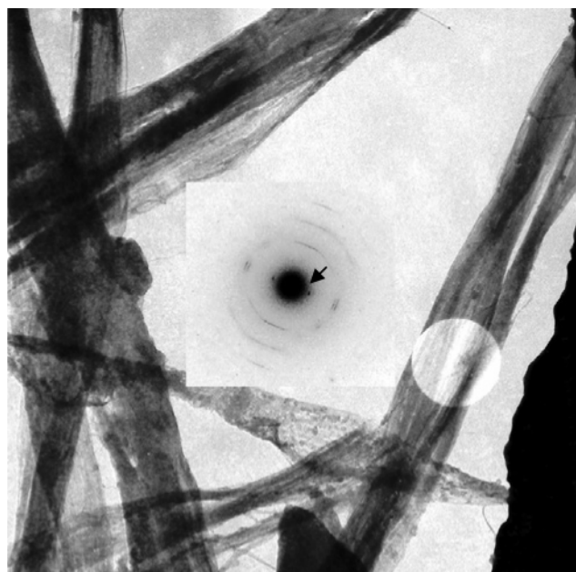
Figure 2. Transmission electron micrograph by diffraction contrast of Lamellibrachia \beta -chitin after heat treatment with acrylic acid. In the middle, a selected area of diffraction from the circled area of 1 \mu\text{m} diameter on the image is shown. Arrow: reflection corresponding to 1.14 nm, which indicates an increased distance between chitin molecular sheets.
