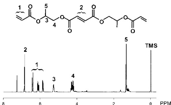
Figure 3. Nuclear magnetic resonance spectra of poly(propylene fumarate) (PPF) and propylene fumarate diacrylate (PFDA).
