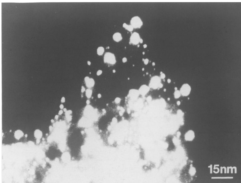
Fig. 1. Z contrast image of Ru particles on a high surface area carbon support.
