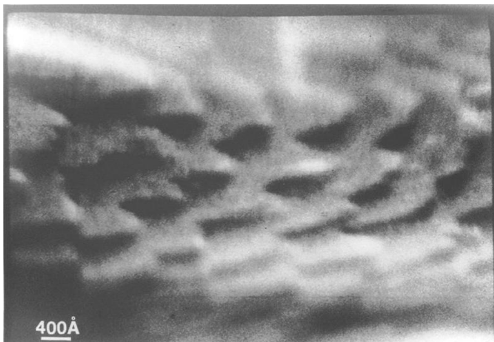
Fig. 4. REM image showing steps approximately 150 Å in height on the surface of a zeolite crystal. The magnification in the y -direction is reduced by about \times 7 relative to that in the x -direction due to the glancing angle of the incident beam.
