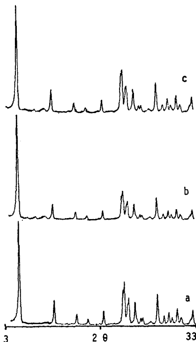
Fig. 3. XRD patterns of sample VPI-5B after a: heating at 960^{\circ}\text{C} under vacuum, b: after heating at 700^{\circ}\text{C} in a flow \text{He/O}_2 , c: sample VPI-5A after heating at 700^{\circ}\text{C} under vacuum, rehydration at ambient conditions and evacuated at 120^{\circ}\text{C} and heated in air at 700^{\circ}\text{C} .
