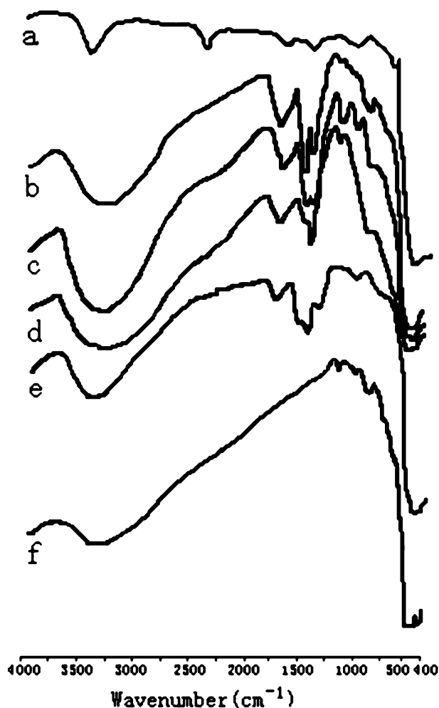
Figure 3. FTIR spectra of samples: (a) ZnO; (b) KF/ZnO without calcination; (c) KF/ZnO calcined at 673 K; (d) KF/ZnO calcined at 773 K; (e) KF/ZnO calcined at 873 K; (f) KF/ZnO calcined at 973 K.
