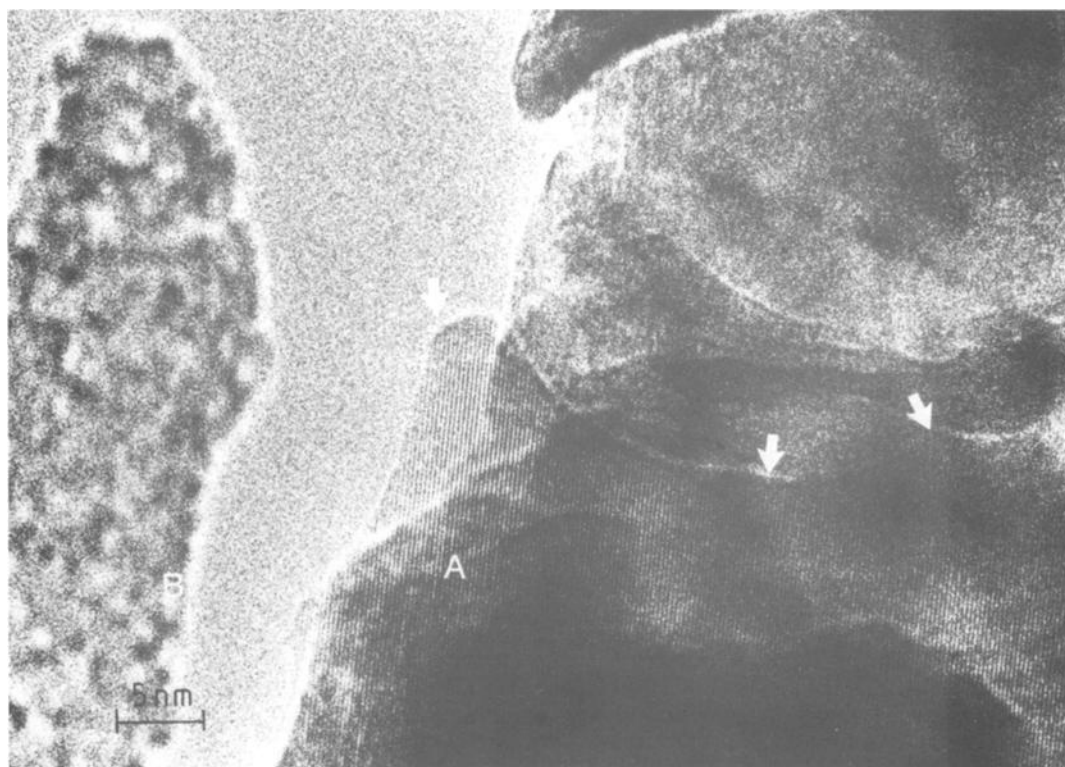
Fig. 8. High resolution TEM image of a single Fe metal platelet.
