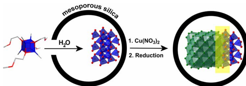
Fig. 1 Schematic representation of the synthetic approach used for the synthesis of Cu–ZnO x model catalysts. The reaction of a special, organometallic precursor, a heterocubane [MeZnOEtOMe] 4 with water results in nanocrystalline ZnO with Wurtzite structure confined
