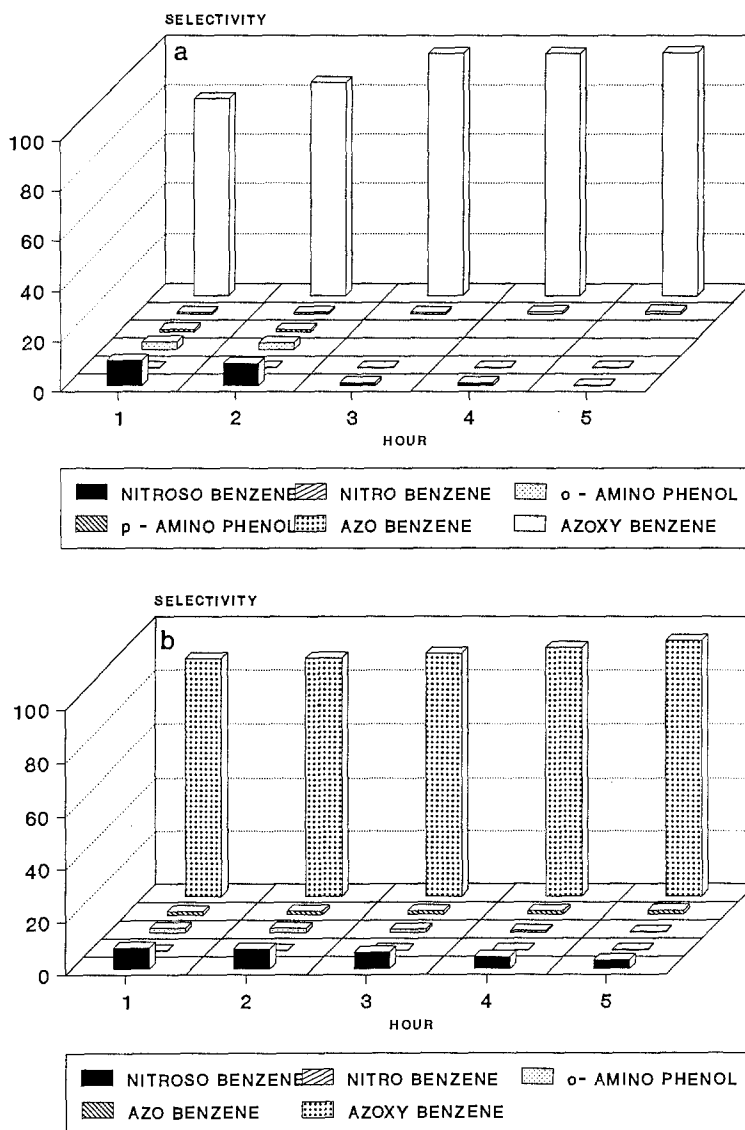
Fig. 1. Influence of mode of addition of H_2O_2 on the oxidation of aniline with TS-1. (a) Addition of H_2O_2 in one lot. (b) Addition over a period of 1 h. (c) Addition over a period of 5 h. (d) Aniline conversion and H_2O_2 selectivity for each mode of addition of H_2O_2 corresponding to (a), (b) and (c), respectively.
