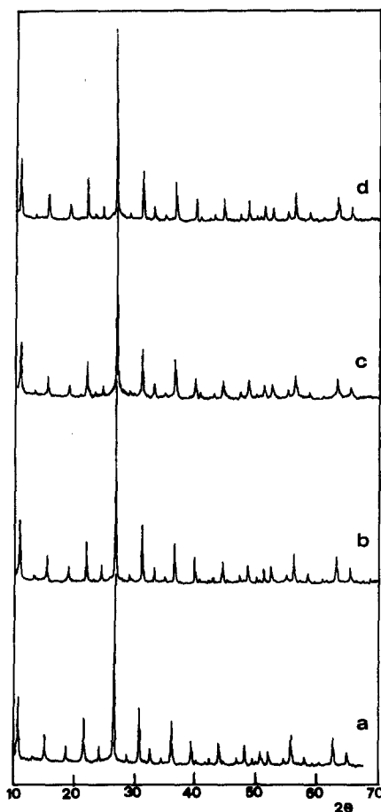
Fig. 1. XRD patterns of the K_1Fe_x samples after calcination at 350°C. (a) x = 0 ; (b) x = 0.5 ; (c) x = 1.0 ; (d) x = 1.5 .
