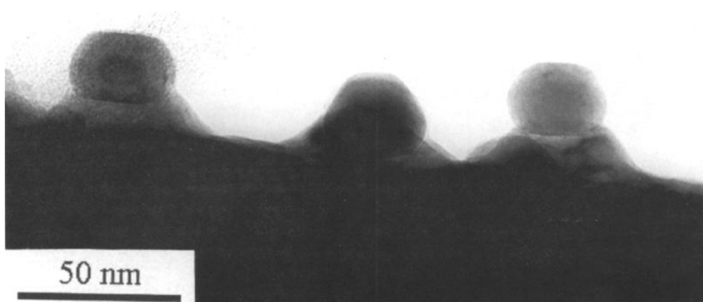
Fig. 5. A TEM image of an \text{La}_4\text{PdO}_7 particle exposed to oxidising atmosphere ( S = 1.1 ) having \text{Pd} particles on its surface.
