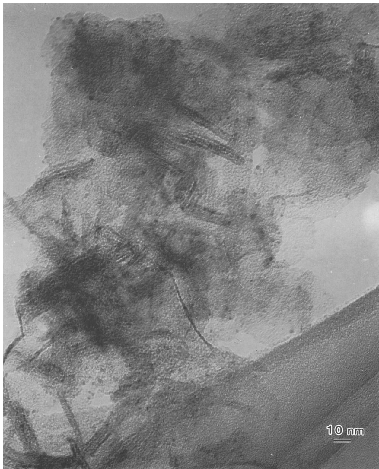
Fig. 5. TEM photograph of aged Au/Mg(OH) 2 . Thin needles of catalyst observed in this photograph are of Mg(OH) 2 crystals viewed from the side. Representative bi-particles are shown circled.
