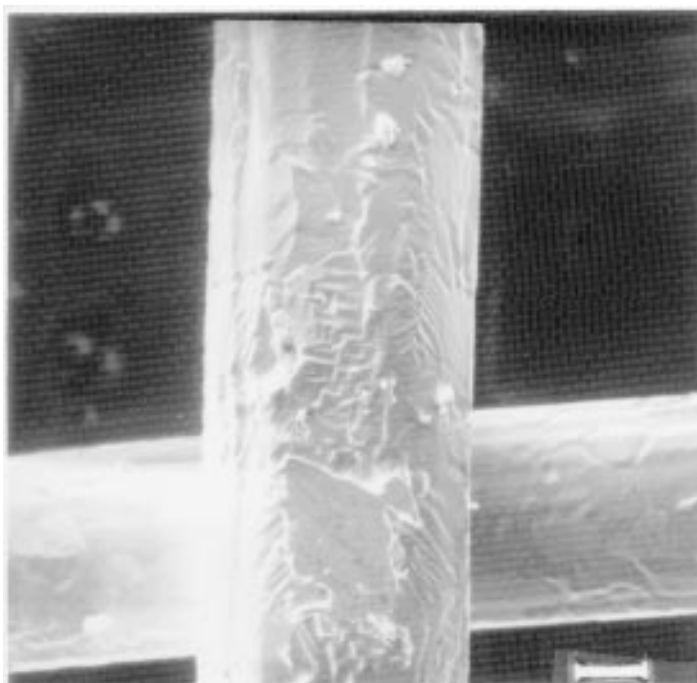
Figure 3. SEM image of the Pt/10% Rh gauze after 8 h on stream. The white bar equals 20 \mu\text{m} .
