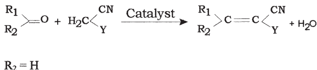
Scheme 1. Knoevenagel condensation of different carbonyl compounds with malononitrile or ethyl cyanoacetate.
