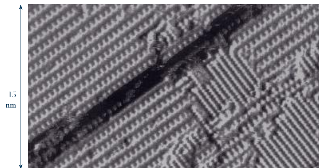
Atomic resolution by STM of nitrogen and oxygen adatoms present at a Cu (110) surface after the oxidation of ammonia. The nitrogen and oxygen adatoms are present in separate phases at right angles to each other (after Carley, Davies & Roberts)
