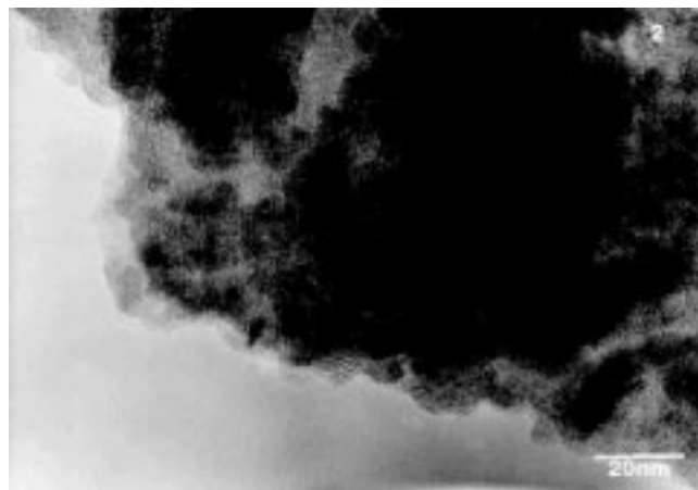
Figure 5. HRTEM/EDX comparable analyses of Cr_5Ti mixed oxides catalyst before and after reaction: (1) fresh and (2) used.
