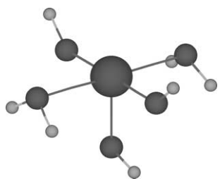
Figure 1. The M(OH)_3(H_2O)_2 cluster used as a model of the active sites.
