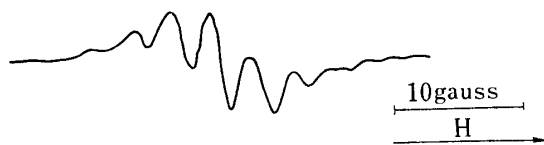
Fig. 7. Electron Spin Resonance Spectrum of 2,7-Dimethyl-3,8-dichlorodibenzo- p -dioxin (X) in conc. Sulfuric Acid with Potassium Nitrate
