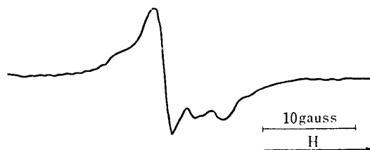
Fig. 4. Electron Spin Resonance Spectrum of 2,7-Dimethyldibenzo- p -dioxin (VI) (soon after the addition of \text{SbCl}_5 )
