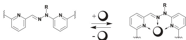
Fig. 3 Conversion of a free linearity unit (left) into a bound helicity inducing unit, a terpy-like site (right), by coordination of a cation.
