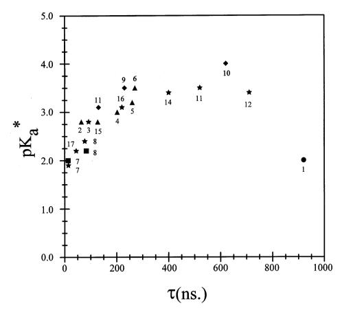
Fig. 1. The  $pK_a^*$  for the different complexes vs. the lifetime of the MLCT state of the unprotonated complex. The numbers adjacent to the individual points refer to the number of the complex in Table 1.
