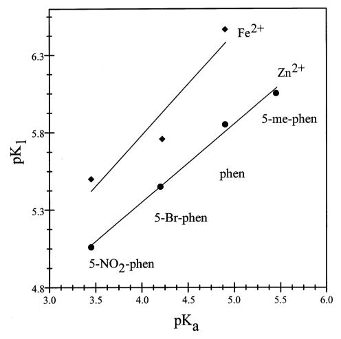
Fig. 3. The dependence of the equilibrium constant for coordination of different phenanthrolines onto Fe(II) and Zn(II) on the  $pK_a$  of the ligand.
